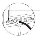
When a command to the parallel printer interface sends a card to the Smart Card Contact Station, the printer connects the Smart Card Contact Station to the female DB-9 connector on the rear of the printer.
